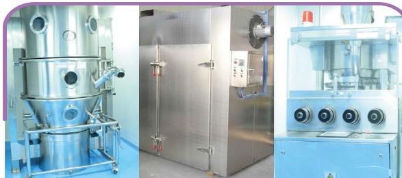
Use of Hi-tech machineries - Fluid Bed Dryer, Multiple Tray Dryer, High Capacity Compression & Filling Machine
